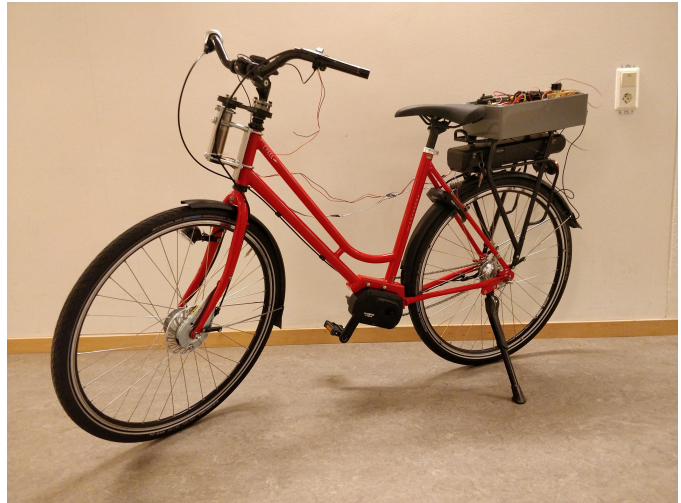
Fig. 1. The bicycle used for the project was a Skeppshult Cyk EL 7. The bike in the picture has been equipped with a steering motor, sensors and other electronics.
